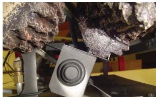
Figure 24A - Installing Front Left Log Side View
